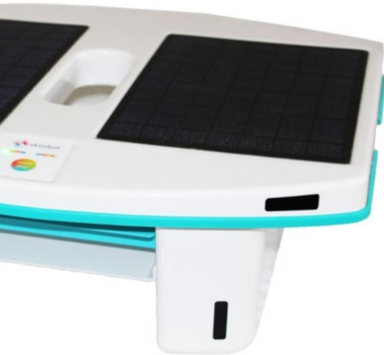
Skimbot has proximity sensors at the front to determine when it's getting close to an obstruction or the edge of the pool. When it nears such an obstacle, the side paddlewheels will rotate at different speeds or in opposite directions in order to steer around the obstacle. Navigation is governed automatically by the software, based on the information it receives from the sensors.
